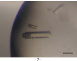
Figure 1 Hexagonal column-shaped crystals of (a) MotY and (b) SeMet-labelled MotY. The scale bar is 0.1 mm in length.
